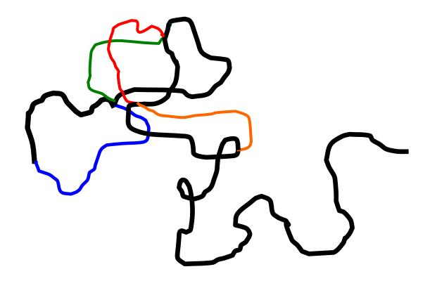
Random walk: (time to move move distance L) = (time per step) x (L/d)<sup>2</sup> steps
