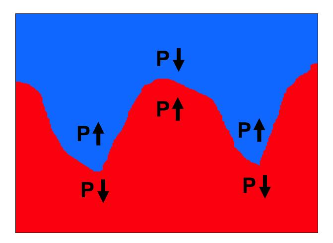
Conservation of energy a.k.a. Bernoulli's Principle → change in mean kinetic energy offset by change in thermal energy (pressure)
